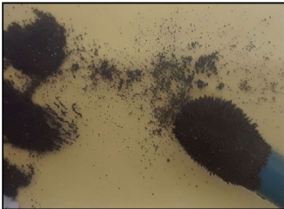
Figure 11: Black sand consisting of magnetite powder and micro-beads, extracted from this heavy sand, bristles in spikes under the effect of a magnetic field (AMC, 2019)
