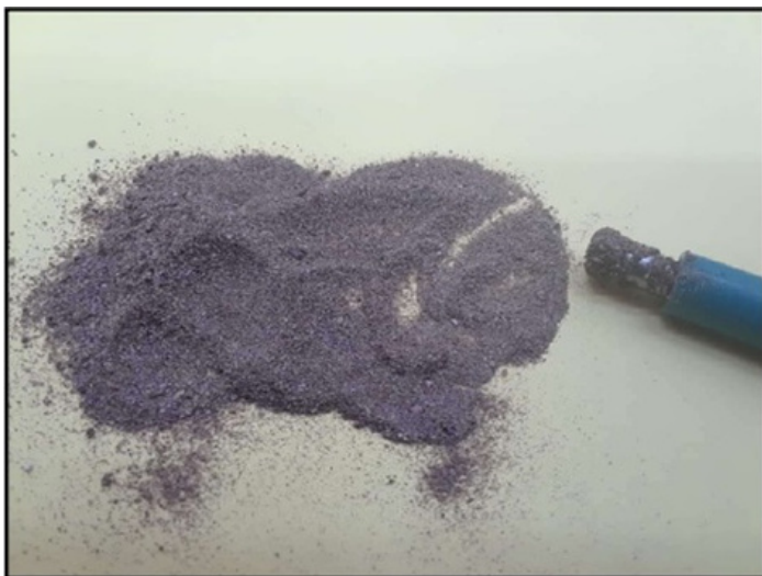
Photo 14: Medium magnetized brown sand, iron (magnetite and hematite) and numerous light grains (quartz and feldspar) (AMC, 2019).
