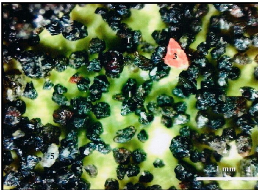
Figure 12: Minerals are shiny and blunt: magnetite minerals (1), hematite (2), olivine, fragments of siliceous rock grains (3) (rhyolite), some rare quartz (4) and feldspar (5) (AMC, 2019)
